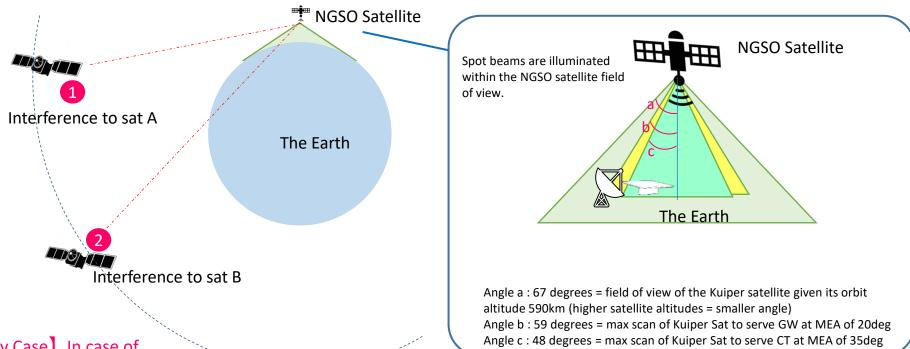
【Satellite Anomaly Case】 In case of anomaly, such as guidance navigation and control (GNC) failure, the Kuiper satellite is designed to go into a power saving mode automatically, for which it will shut off transmissions.
